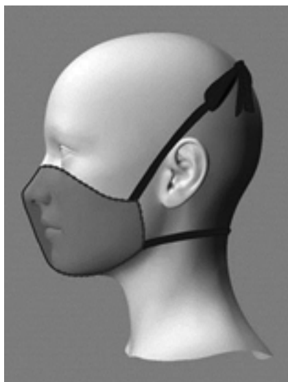
Fig. 1—Face covering covers the user's nose and mouth and makes contact at perimeter (dotted line).
