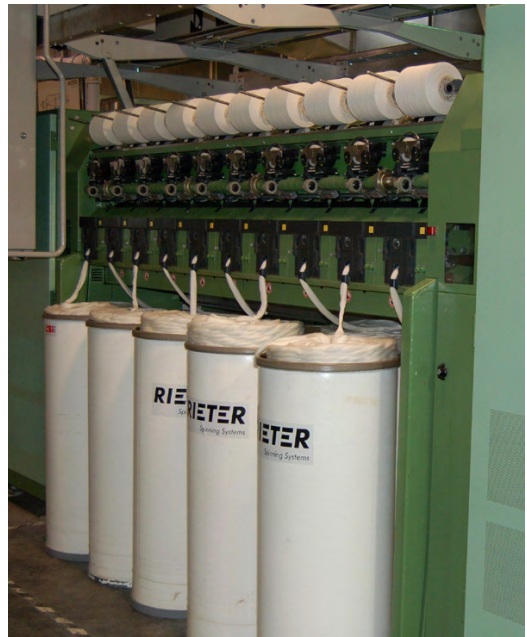
Fig. 3.8. Modern machine spinning of machine-carded cotton fiber roving. Courtesy of North Carolina State University. Used with permission.
