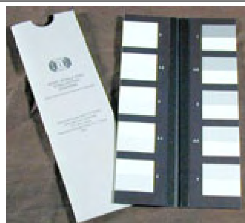
Fig. 13.16. The AATCC Gray Scale for Staining.
