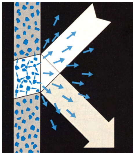
Fig. 3.30. A schematic representation of the absorption and scattering of a light beam in a paint layer. The light beam arrives from the upper right. Some of the light is reflected directly on the surface. Other light is absorbed or scattered by the blue pigment particles. Gall, L., Farbmetrik auf dem Pigmentgebiet , BASF, Ludwigshafen, ca. 1972.
